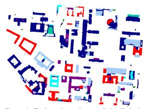
Figure 6: Final result: roof map of the Karlsruhe University (enlarged section approximately 0,8 km x 0,5 km, legend see Figure 4).
